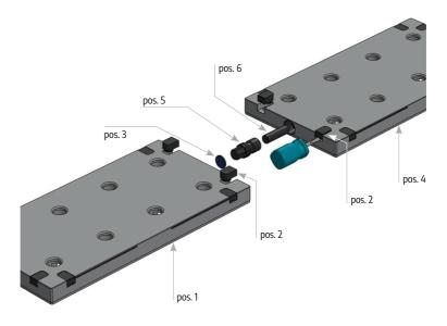
The connecting plate 2, which is to be connected in series (pos. 4), includes a cap for the connectors (pos. 2) as well as the tightening screw (pos. 5) and the actuation bolt (pos. 6), which also need to be removed.
